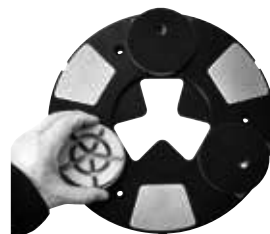
3. Attachment of resin diamonds
