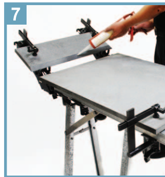
Spread the glue on the mitre of two slabs.
