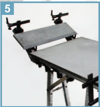
Place the fascia and ensure the two slabs are aligned.
